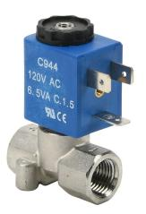
CFA solenoid valve, 3-port (3-way), 2-position, N.C., stainless steel body, Viton seal(s), 1/4in female NPT inlet(s), 1/4in female NPT outlet(s), Cv=0.084, 0 psi minimum operating pressure, 120 VAC operating voltage, 11mm DIN style wiring plug.
