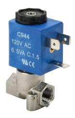
CFA solenoid valve, 3-port (3-way), 2-position, N.C., stainless steel body, Viton seal(s), 1/8in female NPT inlet(s), 1/8in female NPT outlet(s), Cv=0.084, 0 psi minimum operating pressure, 120 VAC operating voltage, 11mm DIN style wiring plug.
