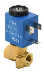
CFA solenoid valve, 3-port (3-way), 2-position, N.C., brass body, Viton seal(s), 1/8in female NPT inlet(s), 1/8in female NPT outlet(s), Cv=0.084, 0 psi minimum operating pressure, 120 VAC operating voltage, 11mm DIN style wiring plug.
