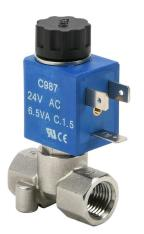
CFA solenoid valve, 2-port (2-way), 2-position, N.O., stainless steel body, Viton seal(s), 1/4in female NPT inlet(s), 1/4in female NPT outlet(s), Cv=0.065, 0 psi minimum operating pressure, 24 VAC operating voltage, 11mm DIN style wiring plug.
