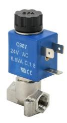
CFA solenoid valve, 2-port (2-way), 2-position, N.O., stainless steel body, Viton seal(s), 1/8in female NPT inlet(s), 1/8in female NPT outlet(s), Cv=0.086, 0 psi minimum operating pressure, 24 VAC operating voltage, 11mm DIN style wiring plug.
