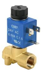
CFA solenoid valve, 2-port (2-way), 2-position, N.O., brass body, Viton seal(s), 1/4in female NPT inlet(s), 1/4in female NPT outlet(s), Cv=0.065, 0 psi minimum operating pressure, 24 VAC operating voltage, 11mm DIN style wiring plug.
