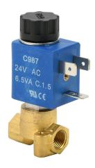
CFA solenoid valve, 2-port (2-way), 2-position, N.O., brass body, Viton seal(s), 1/8in female NPT inlet(s), 1/8in female NPT outlet(s), Cv=0.086, 0 psi minimum operating pressure, 24 VAC operating voltage, 11mm DIN style wiring plug.
