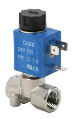
CFA solenoid valve, 2-port (2-way), 2-position, N.O., stainless steel body, Viton seal(s), 1/4in female NPT inlet(s), 1/4in female NPT outlet(s), Cv=0.065, 0 psi minimum operating pressure, 24 VDC operating voltage, 11mm DIN style wiring plug.
