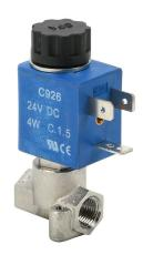
CFA solenoid valve, 2-port (2-way), 2-position, N.O., stainless steel body, Viton seal(s), 1/8in female NPT inlet(s), 1/8in female NPT outlet(s), Cv=0.086, 0 psi minimum operating pressure, 24 VDC operating voltage, 11mm DIN style wiring plug.
