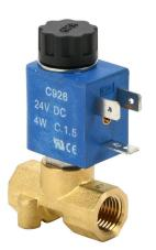
CFA solenoid valve, 2-port (2-way), 2-position, N.O., brass body, Viton seal(s), 1/4in female NPT inlet(s), 1/4in female NPT outlet(s), Cv=0.065, 0 psi minimum operating pressure, 24 VDC operating voltage, 11mm DIN style wiring plug.
