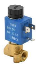
CFA solenoid valve, 2-port (2-way), 2-position, N.O., brass body, Viton seal(s), 1/8in female NPT inlet(s), 1/8in female NPT outlet(s), Cv=0.086, 0 psi minimum operating pressure, 24 VDC operating voltage, 11mm DIN style wiring plug.
