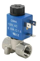
CFA solenoid valve, 2-port (2-way), 2-position, N.O., stainless steel body, Viton seal(s), 1/4in female NPT inlet(s), 1/4in female NPT outlet(s), Cv=0.065, 0 psi minimum operating pressure, 120 VAC operating voltage, 11mm DIN style wiring plug.
