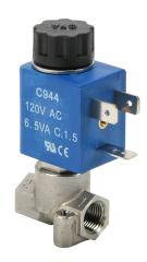
CFA solenoid valve, 2-port (2-way), 2-position, N.O., stainless steel body, Viton seal(s), 1/8in female NPT inlet(s), 1/8in female NPT outlet(s), Cv=0.086, 0 psi minimum operating pressure, 120 VAC operating voltage, 11mm DIN style wiring plug.
