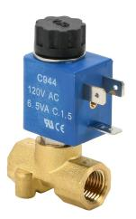
CFA solenoid valve, 2-port (2-way), 2-position, N.O., brass body, Viton seal(s), 1/4in female NPT inlet(s), 1/4in female NPT outlet(s), Cv=0.065, 0 psi minimum operating pressure, 120 VAC operating voltage, 11mm DIN style wiring plug.
