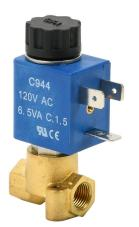
CFA solenoid valve, 2-port (2-way), 2-position, N.O., brass body, Viton seal(s), 1/8in female NPT inlet(s), 1/8in female NPT outlet(s), Cv=0.086, 0 psi minimum operating pressure, 120 VAC operating voltage, 11mm DIN style wiring plug.
