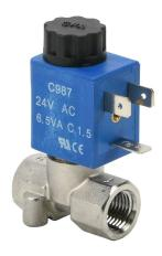
CFA solenoid valve, 2-port (2-way), 2-position, N.C., stainless steel body, Viton seal(s), 1/4in female NPT inlet(s), 1/4in female NPT outlet(s), Cv=0.14, 0 psi minimum operating pressure, 24 VAC operating voltage, 11mm DIN style wiring plug.
