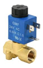
CFA solenoid valve, 2-port (2-way), 2-position, N.C., brass body, Viton seal(s), 1/4in female NPT inlet(s), 1/4in female NPT outlet(s), Cv=0.14, 0 psi minimum operating pressure, 24 VAC operating voltage, 11mm DIN style wiring plug.
