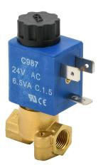
CFA solenoid valve, 2-port (2-way), 2-position, N.C., brass body, Viton seal(s), 1/8in female NPT inlet(s), 1/8in female NPT outlet(s), Cv=0.14, 0 psi minimum operating pressure, 24 VAC operating voltage, 11mm DIN style wiring plug.
