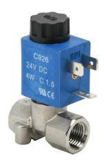
CFA solenoid valve, 2-port (2-way), 2-position, N.C., stainless steel body, Viton seal(s), 1/4in female NPT inlet(s), 1/4in female NPT outlet(s), Cv=0.14, 0 psi minimum operating pressure, 24 VDC operating voltage, 11mm DIN style wiring plug.
