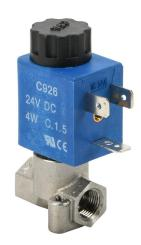
CFA solenoid valve, 2-port (2-way), 2-position, N.C., stainless steel body, Viton seal(s), 1/8in female NPT inlet(s), 1/8in female NPT outlet(s), Cv=0.14, 0 psi minimum operating pressure, 24 VDC operating voltage, 11mm DIN style wiring plug.
