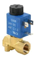
CFA solenoid valve, 2-port (2-way), 2-position, N.C., brass body, Viton seal(s), 1/4in female NPT inlet(s), 1/4in female NPT outlet(s), Cv=0.14, 0 psi minimum operating pressure, 24 VDC operating voltage, 11mm DIN style wiring plug.
