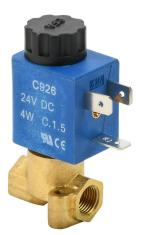
CFA solenoid valve, 2-port (2-way), 2-position, N.C., brass body, Viton seal(s), 1/8in female NPT inlet(s), 1/8in female NPT outlet(s), Cv=0.14, 0 psi minimum operating pressure, 24 VDC operating voltage, 11mm DIN style wiring plug.
