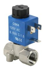
CFA solenoid valve, 2-port (2-way), 2-position, N.C., stainless steel body, Viton seal(s), 1/4in female NPT inlet(s), 1/4in female NPT outlet(s), Cv=0.14, 0 psi minimum operating pressure, 120 VAC operating voltage, 11mm DIN style wiring plug.
