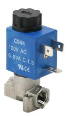
CFA solenoid valve, 2-port (2-way), 2-position, N.C., stainless steel body, Viton seal(s), 1/8in female NPT inlet(s), 1/8in female NPT outlet(s), Cv=0.14, 0 psi minimum operating pressure, 120 VAC operating voltage, 11mm DIN style wiring plug.
