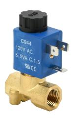
CFA solenoid valve, 2-port (2-way), 2-position, N.C., brass body, Viton seal(s), 1/4in female NPT inlet(s), 1/4in female NPT outlet(s), Cv=0.14, 0 psi minimum operating pressure, 120 VAC operating voltage, 11mm DIN style wiring plug.
