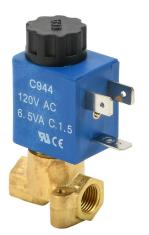
CFA solenoid valve, 2-port (2-way), 2-position, N.C., brass body, Viton seal(s), 1/8in female NPT inlet(s), 1/8in female NPT outlet(s), Cv=0.14, 0 psi minimum operating pressure, 120 VAC operating voltage, 11mm DIN style wiring plug.
