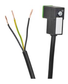
Murrelektronik solenoid valve cable, 9.4mm DIN style molded connector to 3-wire pigtail, 24 VAC/VDC, 18 AWG, PVC jacket, 16.4ft/5m cable length, surge protection, LED indication.
