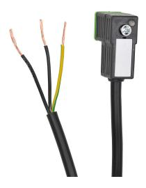
Murrelektronik solenoid valve cable, 9.4mm DIN style molded connector to 3-wire pigtail, 24 VAC/VDC, 18 AWG, PVC jacket, 9.8ft/3m cable length, surge protection, LED indication.
