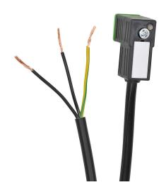
Murrelektronik solenoid valve cable, 9.4mm DIN style molded connector to 3-wire pigtail, 110 VAC/VDC, 18 AWG, PVC jacket, 9.8ft/3m cable length, surge protection, LED indication.
