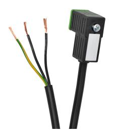
Murrelektronik solenoid valve cable, 9.4mm DIN style molded connector to 3-wire pigtail, 230 VAC/VDC, 18 AWG, PVC jacket, 16.4ft/5m cable length.
