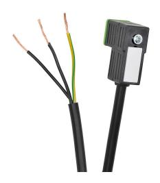
Murrelektronik solenoid valve cable, 9.4mm DIN style molded connector to 3-wire pigtail, 230 VAC/VDC, 18 AWG, PVC jacket, 9.8ft/3m cable length.
