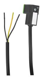
Murrelektronik solenoid valve cable, 8mm DIN 43650 Form C molded connector to 3-wire pigtail, 24 VAC/VDC, 18 AWG, PVC jacket, 16.4ft/5m cable length, surge protection, LED indication.
