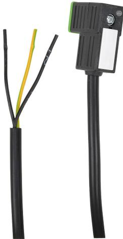
Murrelektronik solenoid valve cable, 8mm DIN 43650 Form C molded connector to 3-wire pigtail, 24 VAC/VDC, 18 AWG, PVC jacket, 16.4ft/5m cable length, surge protection, LED indication.
