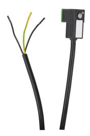
Murrelektronik solenoid valve cable, 8mm DIN 43650 Form C molded connector to 3-wire pigtail, 24 VAC/VDC, 18 AWG, PVC jacket, 9.8ft/3m cable length, surge protection, LED indication.
