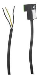
Murrelektronik solenoid valve cable, 8mm DIN 43650 Form C molded connector to 3-wire pigtail, 110 VAC/VDC, 18 AWG, PVC jacket, 16.4ft/5m cable length, surge protection, LED indication.
