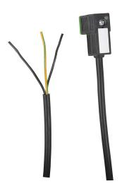
Murrelektronik solenoid valve cable, 8mm DIN 43650 Form C molded connector to 3-wire pigtail, 110 VAC/VDC, 18 AWG, PVC jacket, 9.8ft/3m cable length, surge protection, LED indication.
