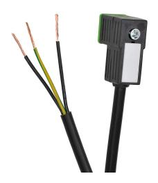
Murrelektronik solenoid valve cable, 8mm DIN 43650 Form C molded connector to 3-wire pigtail, 230 VAC/VDC, 18 AWG, PVC jacket, 16.4ft/5m cable length.
