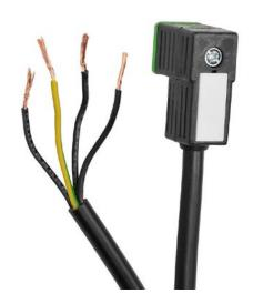
Murrelektronik transmitter cable, 8mm DIN 43650 Form C molded connector to 4-wire pigtail, 230 VAC/VDC, 18 AWG, PVC jacket, 16.4ft/5m cable length.
