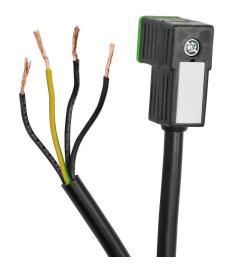
Murrelektronik transmitter cable, 8mm DIN 43650 Form C molded connector to 4-wire pigtail, 230 VAC/VDC, 18 AWG, PVC jacket, 16.4ft/5m cable length.
