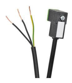
Murrelektronik solenoid valve cable, 8mm DIN 43650 Form C molded connector to 3-wire pigtail, 230 VAC/VDC, 18 AWG, PVC jacket, 9.8ft/3m cable length.
