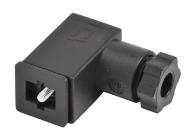
NITRA field wireable solenoid valve connector, 8mm DIN 43650 Form C molded connector, 230 VAC/VDC, 16-12 AWG, accepts cable diameter size 0.20-0.24in.
