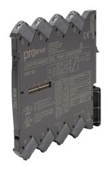
ProSense temperature transmitter, isolated, RTD or thermocouple input, deg C or deg F, current output, 5.5-35 VDC loop powered operating voltage, 35mm DIN rail mount, screw terminals.
