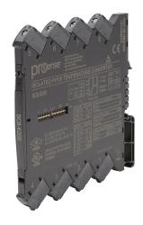
ProSense temperature transmitter, isolated, RTD input, deg C or deg F, current or voltage output, 24 VDC nominal operating voltage, 35mm DIN rail mount, screw terminals.
