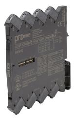
ProSense temperature transmitter, non-isolated, RTD input, deg C or deg F, current output, 3.3-35 VDC loop powered operating voltage, 35mm DIN rail mount, screw terminals.
