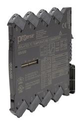
ProSense temperature transmitter, isolated, thermocouple input, deg C or deg F, current or voltage output, 24 VDC nominal operating voltage, 35mm DIN rail mount, screw terminals.
