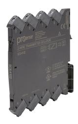
ProSense signal conditioner, isolated, current transmitter input, current output, 6-35 VDC loop powered operating voltage, 35mm DIN rail mount, screw terminals.
