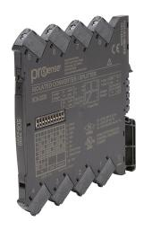
ProSense signal conditioner, isolated, current or voltage input, (2) current or voltage output, 24 VDC nominal operating voltage, 35mm DIN rail mount, screw terminals.
