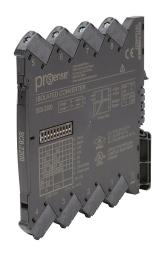
ProSense signal conditioner, isolated, current or voltage input, current or voltage output, 24 VDC nominal operating voltage, 35mm DIN rail mount, screw terminals.
