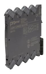
ProSense signal conditioner, (2) isolated channels, current input, current output, 6-35 VDC loop powered operating voltage, 35mm DIN rail mount, screw terminals.
