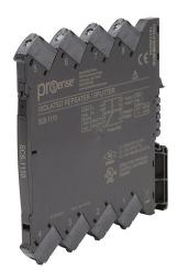
ProSense signal conditioner, isolated, current input, (2) current output, 24 VDC nominal operating voltage, 35mm DIN rail mount, screw terminals.
