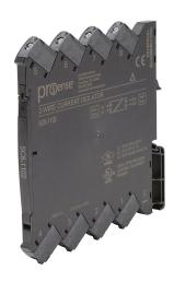
ProSense signal conditioner, isolated, current input, current output, 6-35 VDC loop powered operating voltage, 35mm DIN rail mount, screw terminals.
