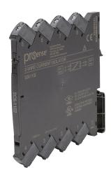
ProSense signal conditioner, isolated, current input, current output, 6-35 VDC loop powered operating voltage, 35mm DIN rail mount, screw terminals.
