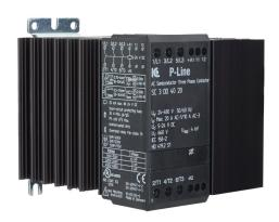
Eltwin SC3 series solid state contactor, 20A, (3) N.O. SCR switched power poles, 24-480 VAC (50/60Hz) operating voltage, 5-24 VDC coil voltage.
